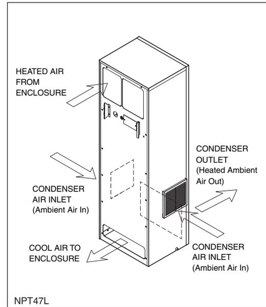
Any enclosure moisture accumulated on the evaporator coil is collected in the condensate tray and removed through the drain tube to the condensate evaporator. Condensate evaporates in the condensate evaporator and is released to the ambient air by the condenser impeller.
