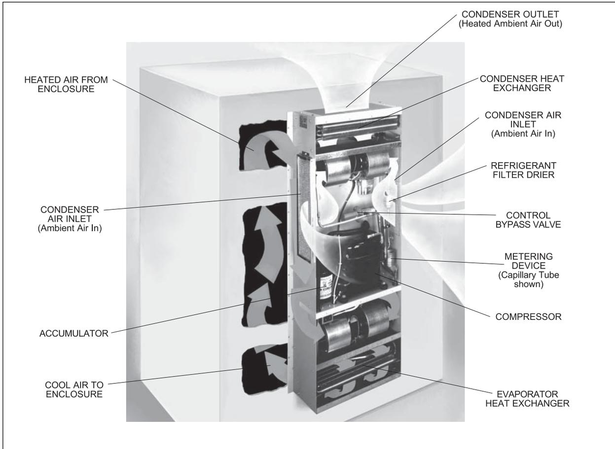
Kooltronic Air Conditioners are required when the equipment operating temperature must be kept near or lower than the ambient room temperature, and/or the cabinet must be sealed from dust, fumes, oil, corrosives and other contaminants. This Air Conditioner utilizes a “Closed-Loop Cooling System” to ensure optimum performance of the installed components.
