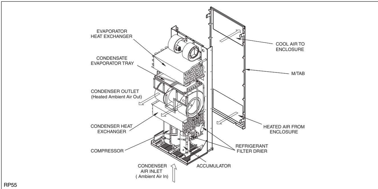
Kooltronic Air Conditioners are required when the equipment operating temperature must be kept near or lower than the ambient room temperature, and/or the cabinet must be sealed from dust, fumes, oil, corrosives and other contaminants. This Air Conditioner utilizes a "Closed-Loop Cooling System" to ensure optimum performance of the installed components.
