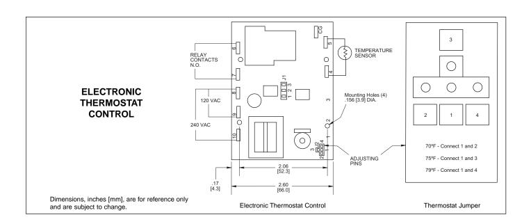
The Low Temperature Thermostat has a test start relay. When the air conditioner is turned on it will run constantly for the first 15 minutes regardless of external temperatures. Afterwards, if the entering evaporator air temperature is lower than the thermostat set point, the compressor and condenser blower will stop, and the thermostat will begin to control the air conditioner.
