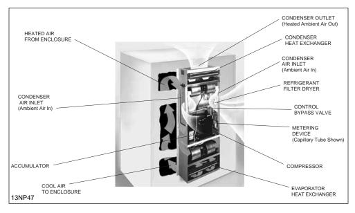
components from the environment. The external system uses circulating ambient air or water to discharge the heat removed from the electronics. The heat is dissipated from the enclosure by means of the vapor compression refrigeration cycle. This takes place in a hermetically-sealed refrigeration system, utilizing either an air-cooled or water-cooled condenser heat exchanger. The warm air inside the enclosure is drawn through the evaporator coil where it is cooled, dehumidified and returned.
