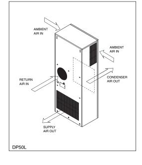
the condensate evaporator and is released to the ambient air by the condenser impeller.
