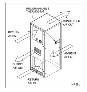
The heat removed through the evaporator coil is transferred by the compressed refrigerant to the condenser coil. Ambient air is then passed through the condenser coil, where it absorbs the heat and is then discharged to the environment.
