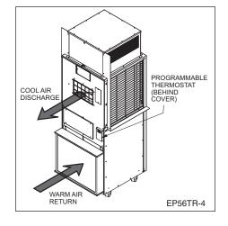
The heat removed through the evaporator coil is transferred by the compressed refrigerant to the condenser coil. Ambient air is then passed through the condenser coil, where it absorbs the heat and is then discharged to the environment.
