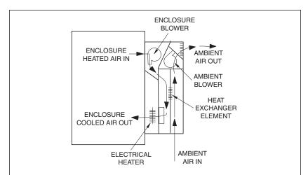
The heater option includes the electrical heater, ambient blower, bimetal thermostat, heater thermostat and limiter thermostat. All of the thermostats are installed in the discharged enclosure air stream. When the enclosure discharge air goes below 70°F, the ambient blower thermostat shuts off the ambient blower. When the enclosure discharge air goes above 85°F, the ambient blower thermostat turns on the ambient blower.
