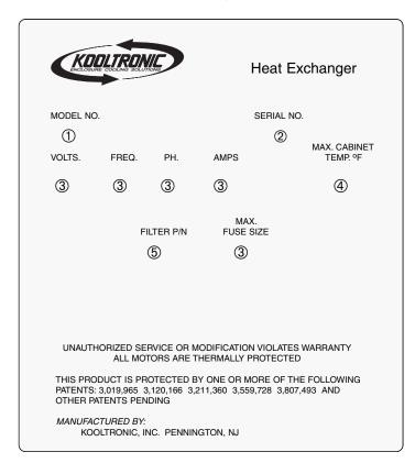
Each Kooltronic Heat Exchanger includes an identification nameplate. This nameplate provides:
