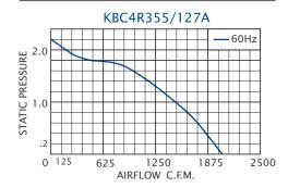
Airflow vs. static pressure curve is shown for 60 Hz input (solid line). Static pressure is in inches of water.
