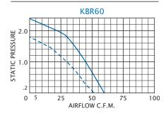
Airflow vs. static pressure curves are shown for 60 Hz and 50 Hz (broken line) inputs. Static pressure is in inches of water.
