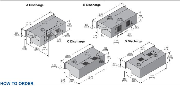
Specify model number, adding discharge suffix A, B, C or D. Example: KPL729A. For 230 VAC operation, add a 2 after the K. Example: K2PL729A.
