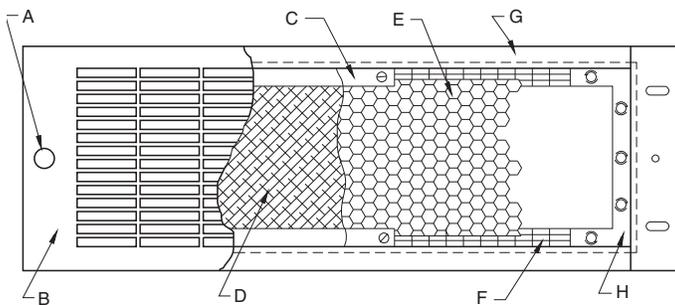
**EMI-SHIELDED FILTER-GRILLE ASSEMBLIES:** (A) Captive Thumbnut, (B) Grille, (C) Plated Steel Retainer Frame, (D) Aluminum Filter, (E) Honeycomb, (F) EMI Gasket (Plated knitted wire mesh), (G) EMI Frame (Plated steel rear surface), (H) Plated steel surface.
