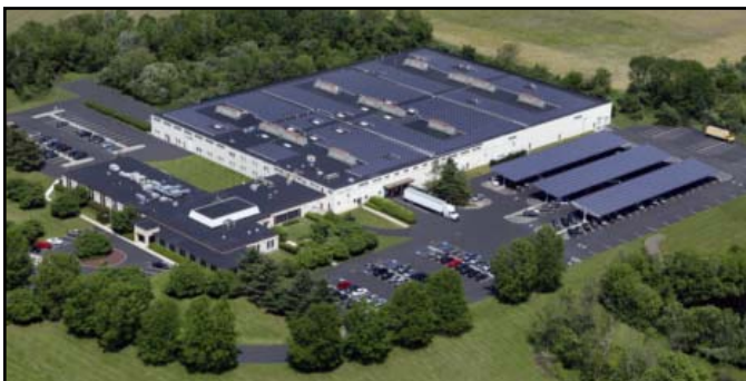
Kooltronic, Inc. Corporate Headquarters, showing approximately 4,000 solar panels in roof top array and parking lot canopies, which provide the facility with 90% of its energy requirements on any given day.
