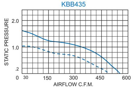
Airflow vs. static pressure curves are shown for 60 Hz and 50 Hz (broken line) inputs. Static pressure is in inches of water.
