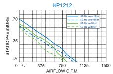
Airflow vs. static pressure curves are shown for 60 Hz (solid line) inputs and 50 Hz (broken line) inputs. Static pressure is in inches of water.
