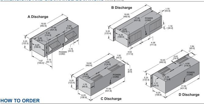
Specify model number, adding discharge suffix A, B, C or D. Example: KP529A. For 230 VAC operation, add a 2 after the K. Example: K2P529A kp529.qxd (8/1/23) (CDR: 20498) Dimensions, inches [mm], are for reference only and subject to change.
