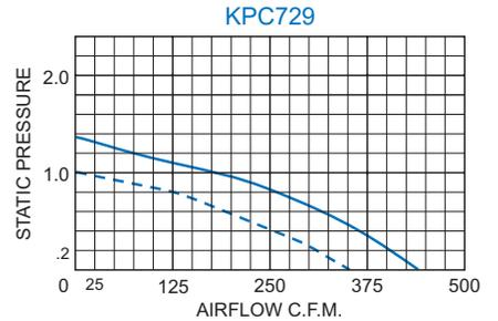
Airflow vs. static pressure curves are shown for 60 Hz (solid line) and 50 Hz (broken line) inputs. Static pressure is in inches of water.
