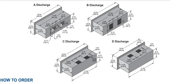
Specify model number, adding discharge suffix A, B, C or D. Example: KPR877A. Unavailable in 230 VAC.
