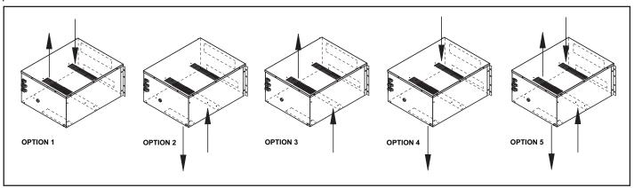
The standard Kooltronic Rack Mount Air Conditioner evaporator airflow is Option 1. In order to convert Option 1 to any of the other options the two cutout covers installed on the unit bottom have to be removed, and installed on the appropriate cutouts. Option 5 is achieved by totally removing the cutout covers.
