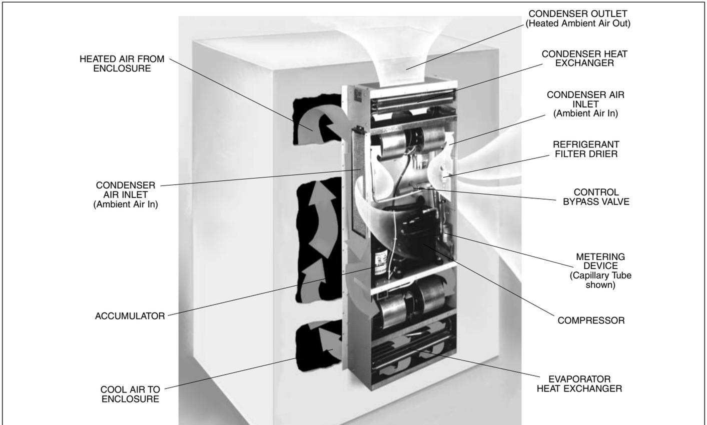
Kooltronic Air Conditioners are required when the equipment operating temperature must be kept near or lower than the ambient room temperature, and/or the cabinet must be sealed from dust, fumes, oil, corrosives and other contaminants. This Air Conditioner utilizes a "Closed-Loop Cooling System" to ensure optimum performance of the installed components.
