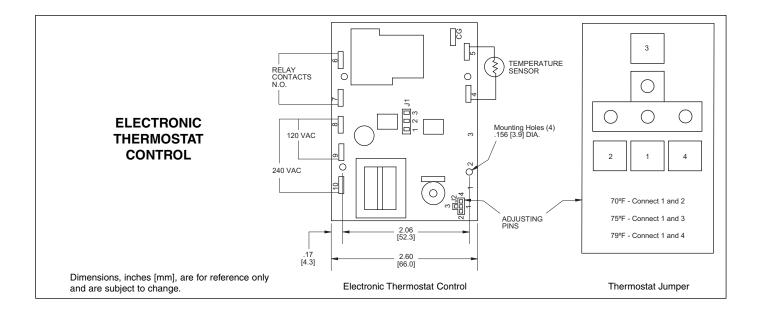
The Low Temperature Thermostat has a test start relay. When the air conditioner is turned on it will run constantly for the first 15 minutes regardless of external temperatures. Afterwards, if the entering evaporator air temperature is lower than the thermostat set point, the compressor and condenser blower will stop, and the thermostat will begin to control the air conditioner.
