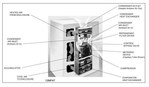
components from the environment. The external system uses circulating ambient air or water to discharge the heat removed from the electronics. The heat is dissipated from the enclosure by means of the vapor compression refrigeration cycle. This takes place in a hermetically-sealed refrigeration system, utilizing either an air-cooled or water-cooled condenser heat exchanger. The warm air inside the enclosure is drawn through the evaporator coil where it is cooled, dehumidified and returned.
