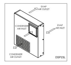
Any enclosure moisture accumulated on the evaporator coil is collected in the condensate tray and removed through the drain tube to the condensate evaporator. Condensate evaporates in the condensate evaporator and is released to the ambient air by the condenser impeller.
