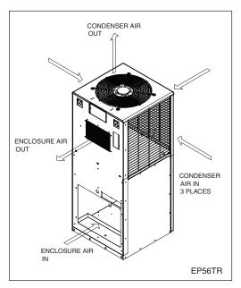
The heat removed through the evaporator coil is transferred by the compressed refrigerant to the condenser coil. Ambient air is then passed through the condenser coil, where it absorbs the heat and is then discharged to the environment.
