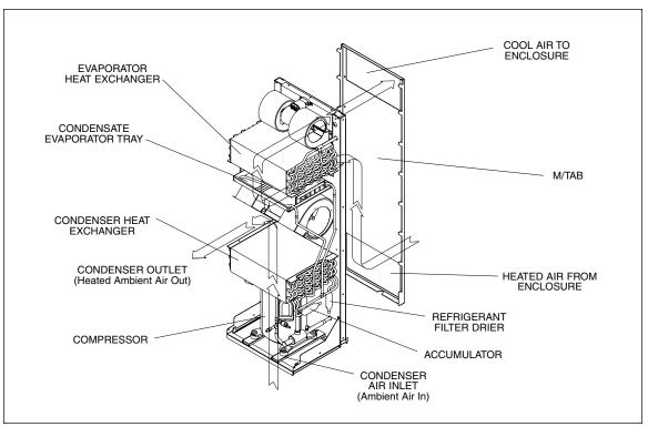
Kooltronic Air Conditioners are required when the equipment operating temperature must be kept near or lower than the ambient room temperature, and/or the cabinet must be sealed from dust, fumes, oil, corrosives and other contaminants. This Air Conditioner utilizes a "Closed-Loop Cooling System" to ensure optimum performance of the installed components.
