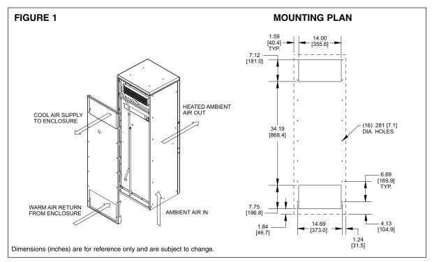
Kooltronic Air Conditioners have been engineered to be installed easily. To avoid damaging your Air Conditioner, please read the following information before installation:
