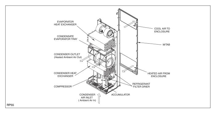
Kooltronic Air Conditioners are required when the equipment operating temperature must be kept near or lower than the ambient room temperature, and/or the cabinet must be sealed from dust, fumes, oil, corrosives and other contaminants. This Air Conditioner utilizes a "Closed-Loop Cooling System" to ensure optimum performance of the installed components.
