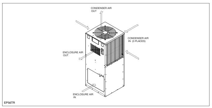
Kooltronic Air Conditioners are required when the equipment operating temperature must be kept near or lower than the ambient room temperature, and/or the cabinet must be sealed from dust, fumes, oil, corrosives and other contaminants. These Air Conditioners utilize a "Closed-Loop Cooling System" to ensure optimum performance of the installed components.
