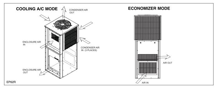
Kooltronic Air Conditioners are required when the equipment operating temperature must be kept near or lower than the ambient room temperature, and/or the cabinet must be sealed from dust, fumes, oil, corrosives and other contaminants. These air conditioners utilize a "Closed-Loop Cooling System" to ensure optimum performance of the installed components.
