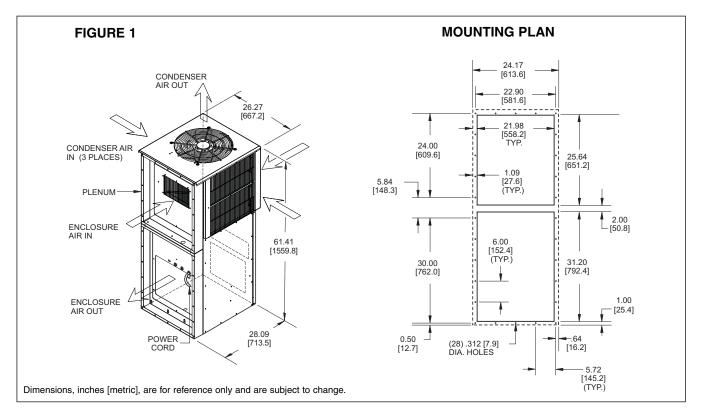
Kooltronic Air Conditioners have been engineered to be easily installed. To avoid damaging your air conditioner, please read the following information before installation:
