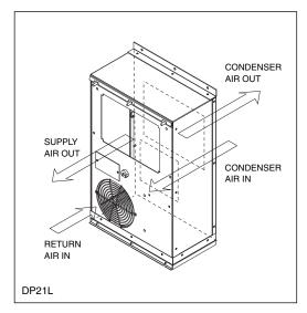
Any enclosure moisture accumulated on the evaporator coil is collected in the condensate tray and removed through the drain tube to the condensate evaporator. Condensate evaporates in the condensate evaporator and is released to the ambient air by the condenser impeller.
