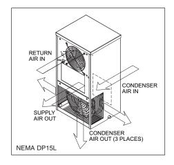
below 40°F the heater will engage. The contact points of the alarm thermostat are normally closed. If the entering evaporator air temperature exceeds 130°F the alarm thermostat contacts open, and when the temperature drops below 130°F the contacts close.
