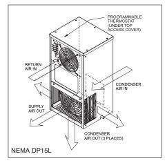
Any enclosure moisture accumulated on the evaporator coil is collected in the condensate tray and removed through the drain tube to the condensate evaporator. Condensate evaporator and is released to the ambient air by the condenser impeller.
