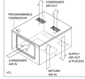
Any enclosure moisture accumulated on the evaporator coil is collected in the condensate tray and removed through the drain tube to the
