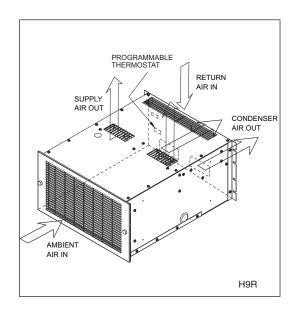
The heat removed through the evaporator coil is transferred by the compressed refrigerant to the condenser coil. Ambient air is then passed through the condenser coil, where it absorbs the heat and is then discharged to the environment.
