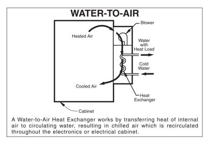
Water-to-Air systems are easy to install and usually require minimum maintenance. The water used must be reasonably clean and cold enough to ensure proper operation of the cooling system under the most severe anticipated conditions. In some cases, if sufficiently cold water is available, below-ambient-temperature cooling can be achieved.
