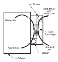
In an Air-to-Air Heat Exchanger, heat from air surrounding the components is removed by a specially designed heat transfer element before being routed back into the enclosure.
