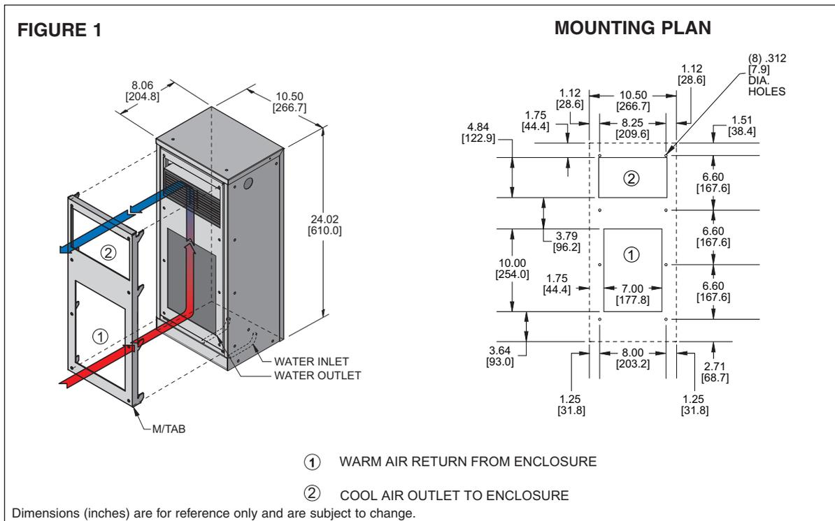
Kooltronic Heat Exchangers have been engineered to be installed easily. To avoid damaging your Heat Exchanger, please read the following information before installation:
