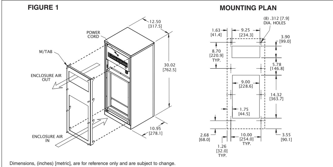
Kooltronic Heat Exchangers have been engineered to be installed easily. To avoid damaging your Heat Exchanger, please read the following information before installation:
