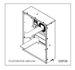
Any enclosure moisture accumulated on the evaporator coil is collected in the condensate tray and removed through the drain tube to the condensate evaporator. Condensate evaporates in the condensate evaporator and is released to the ambient air by the condenser impeller.
