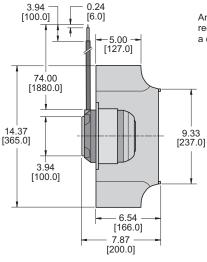
An inlet ring, which must be installed by the customer, is recommended for optimum performance. This unit requires a capacitor which must be connected by the customer.
