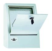
These indoor/outdoor Filter Fan and Exhaust Packages are used in enclosures to dissipate heat harmful to sensitive electronic components. The fans feature a filter that is easily changed by opening the lockable door of the outdoor hood. IP55 protection is reached by the specially-designed hood and the use of special filters. The plastic casing is impact-resistant, weather-proof and UV resistant.
