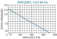
Airflow vs. static pressure curves are shown for 60 Hz and 50 Hz (broken line) inputs.
