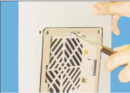
**Step 4.** Clamp the elastic hooks (on the two sides and at the top) by pushing at the base. In case of difficulty, snap in by using a screw driver.
