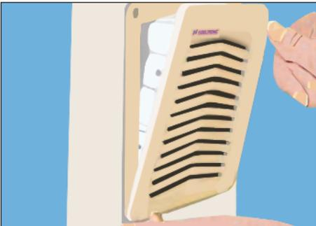
**Step 5.** Put the filter media in the louvered cover (the less dense side of the filter should be facing the air inlet side) and then insert the cover into the base.
