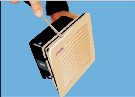
**Step 2.** Remove the louvered cover and filter media from the base by using a screw driver in the slots provided on the edge of the cover.
