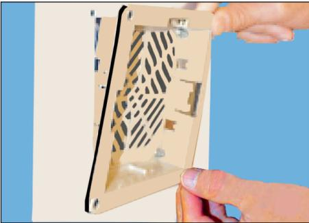
**Step 3.** Insert the base into the mounting hole. Tip the base forward and carefully clamp the fixed hook at the bottom. Note: the positions "TOP" and "BOTTOM" are marked on the base and on the louvered cover.
