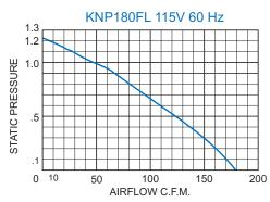
Airflow vs. static pressure curve is shown for 60 Hz (solid line) inputs. Static pressure is in inches of water.
