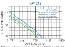
Airflow vs. static pressure curves are shown for 60 Hz (solid line) inputs and 50 Hz (broken line) inputs. Static pressure is in inches of water.
