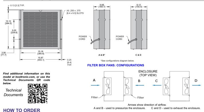
FANS: Specify model number, adding configuration suffix A, B, C or D. Example: KP1212A. Unavailable in 230 VAC. ACCESSORIES: Specify model number.
