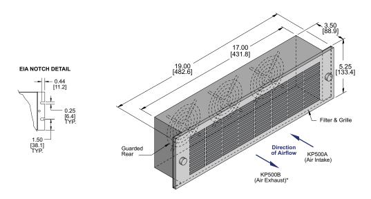
\*For exhaust applications, filter may be removed and used at air intake.
