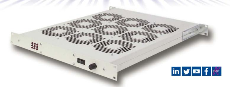
The Kooltronic Kooltray II, with its 1¾" height, is designed to fit under card racks or near heat-producing sources. Standard units are available in 1, 2, or 3 row models. Optional features include thermal fan speed control, fan failure indication and alarm output, DC power supply and filtered fan tray.
