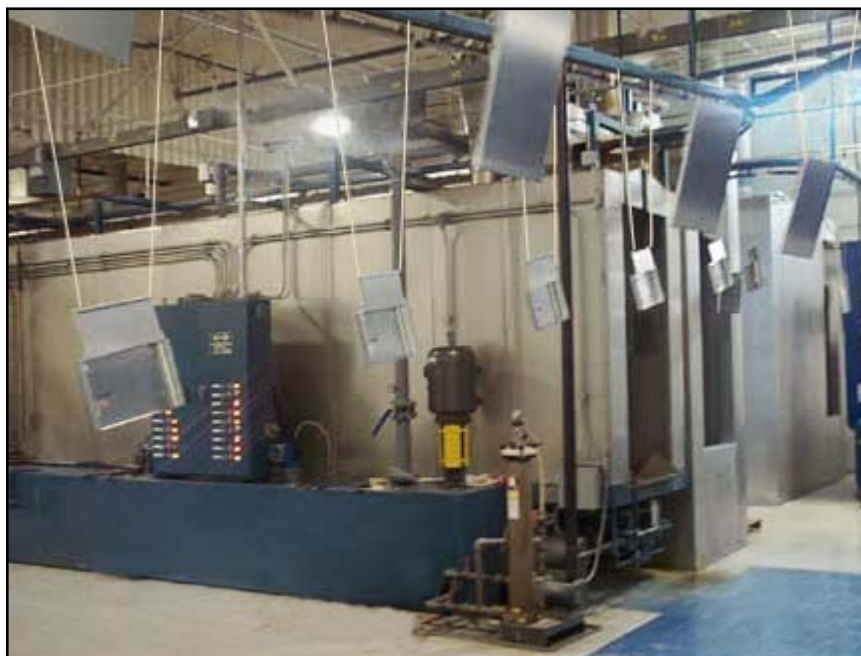
The automated wash system and dry-off oven.
