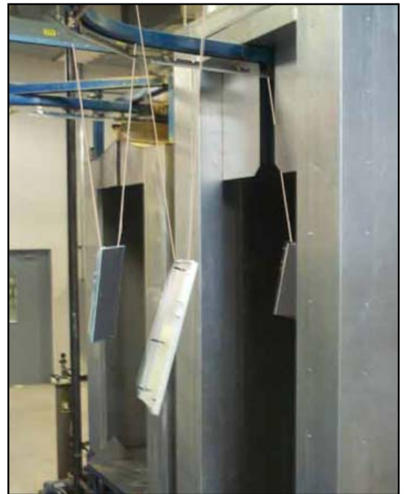
Parts exiting the water dry-off oven.
