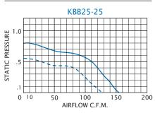
Airflow vs. static pressure curves are shown for 60 Hz (solid line) and 50 Hz (broken line) inputs. Static pressure is in inches of water.
