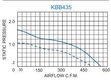
Airflow vs. static pressure curves are shown for 60 Hz and 50 Hz (broken line) inputs. Static pressure is in inches of water.
