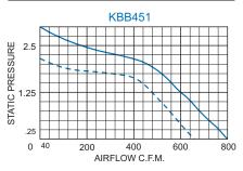
Airflow vs. static pressure curves are shown for 60 Hz and 50 Hz (broken line) inputs. Static pressure is in inches of water.
