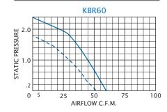
Airflow vs. static pressure curves are shown for 60 Hz (solid line) and 50 Hz (broken line) inputs. Static pressure is in inches of water.
