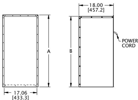
UNIT MUST BE 12" [300mm] MINIMUM ABOVE FLOOR FOR FILTER ACCESS
