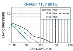
Airflow vs. static pressure curve is shown for 60 Hz inputs. Static pressure is in inches of water.
